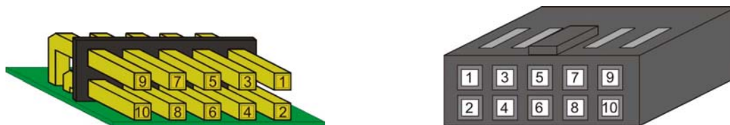
Figure 1: Lumina / SR5 ccTalk Connector
