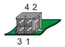
In order to maintain compatibility with earlier versions of Paylink, the pin allocation of this connector is as shown in the diagram to the left.
