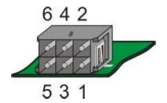
In order to maintain compatibility with earlier versions of Paylink, the pin allocation of this connector is as shown in the diagram to the left.
